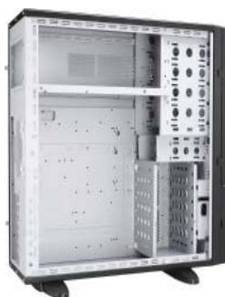
12 drive slots and long cables for easy installation and extension
