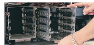
2 removable cages for 8 rubber supported cooled hard disks
