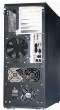
Main board is upside down! PCI-slots on top and the power supply on the bottom
