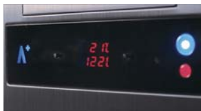
Controller for 4 fans with temperature and fan-speed display the front
