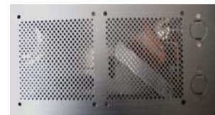
2 x 120 mm fan/ radiator holes and 2 x water tube holes on top
