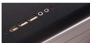
2 x USB 2.0, 2 x Audio connectors and 1 x Firewire on top
